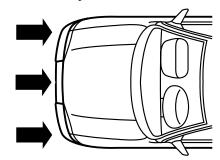
cause activation. Driver and passenger airbags are designed to inflate in frontal and near-frontal collisions, not rollover, side-impact, or rear-impacts unless the collision causes sufficient longitudinal deceleration.
